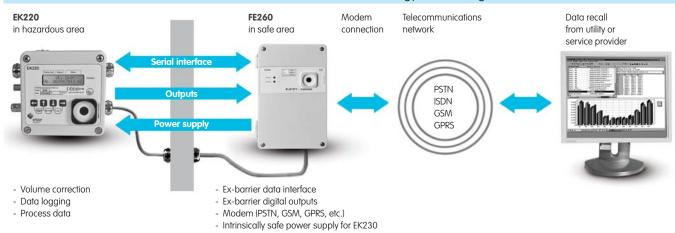
The Ex-barrier of the serial interface and the pulse outputs of the volume corrector is provided by function extension unit FE260. In addition, the intrinsically safe power supply of the volume corrector is guaranteed. The unit's modular concept allows the use of a modem for data communication or an interface for connection to other devices.
